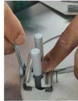
D. REMOVE THE FIXED PORCELAIN CLAMP SCREW
