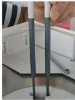
F. REMOVE THE HEATING ELEMENT THAT NEEDS TO BE REPIACED
