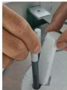
E. REMOVE THE ALUMINA SPACER
