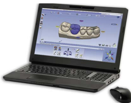
FIG. 14.3 Software (PlanCAD) for the visualization of the scanned data and design of restorations. (Courtesy Planmeca, Roselle, IL.)
