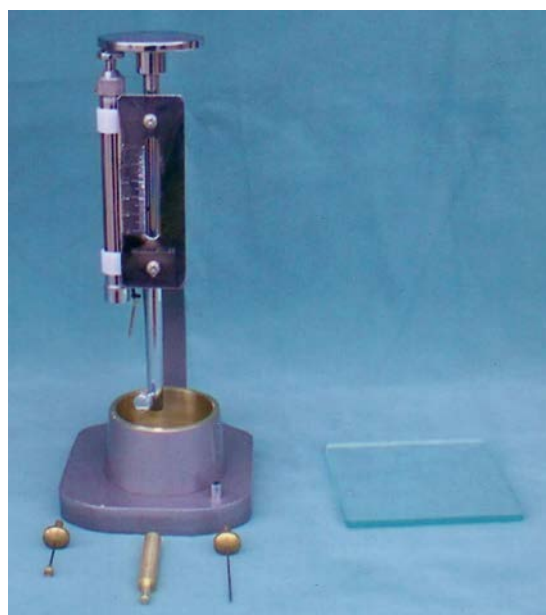
FIG. 5.13 Vicat penetrometer used to determine initial setting time of gypsum products.
