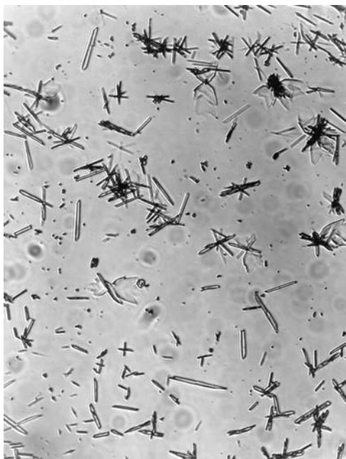
FIG. 12.20 Crystals of model plaster.
