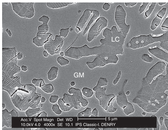
FIG. 11.13 Scanning electron micrograph showing the microstructure of feldspathic porcelain for metal-ceramic restorations. GM, Glassy matrix; LC, leucite crystal.
