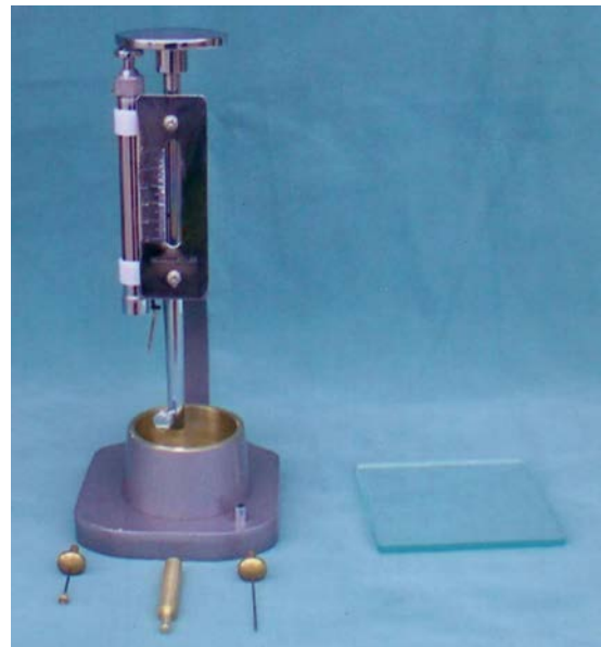
FIG. 12.16 Vicat penetrometer used to determine setting time of impression materials and other restorative materials.
