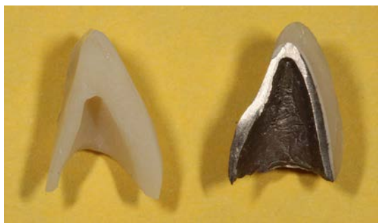
FIG. 11.1 Cutaways of all-ceramic crown (left) and porcelain fused to metal crown (right). (Courtesy Dr. Charles Mark Malloy, Portland, OR.)
