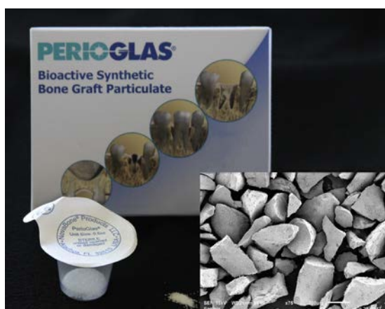
FIG. 16.5 Bioactive glasses are receiving increased attention because of their surface bioactivity. Shown here is PerioGlas (original magnification \times 75 for inset image). (Courtesy John C. Mitchell, Midwestern University College of Dental Medicine-Arizona, Glendale, AZ.)
