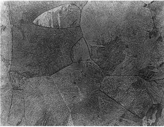
FIG. 10.12 Microstructure of as-cast Ti-6Al-4V.
